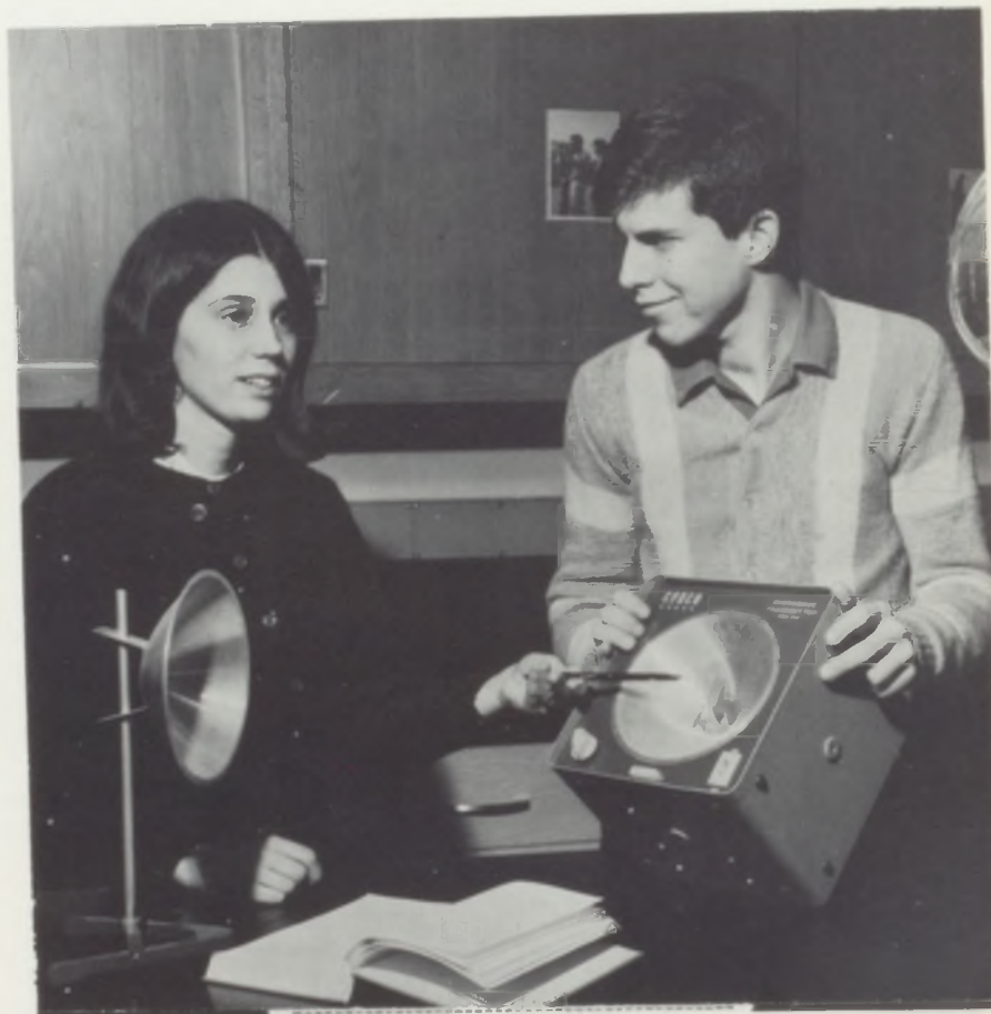
Linda Verbeck and Gene Thrasher demonstrate the use of micro-waves with the transmitter and parabolic reflector, a miniature version of the kinds used in coast-to-coast TV hookups.
